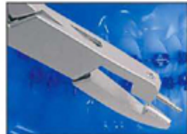
EM-7122 Omega Loop forming pliers with replaceable 440 stainless steel tip, three step tip has 1.14, 1.52 and 1.91mm diameters
